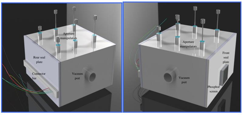
Two views of the outside of the basic experimental chamber which houses all of the major instruments for analysis of the results of both EVO action and its effect on nearby material. The container is made from cast alumina ceramic and then glazed. Of all the components in this proposal, this unit is the one that is modified more often than any other.
