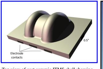
Top view of cast ceramic ITMS shell showing electrode contacts and basic dimension
