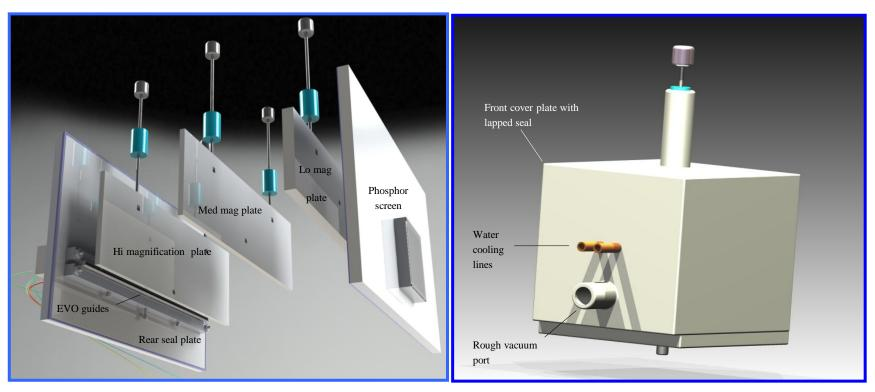
Inside view of the experimental chamber showing one particular experiment used to determine the properties of material vaporized by an impacting EVO. Various degrees of magnification can be set for analysis by manipulating the apertures.
