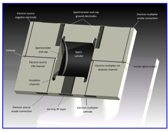
View of active side of cast ceramic ITMS showing electron multipliers and spectrometer cylinder. Two similar plates are assembled to form a complete spectrometer. Several of these small mass spectrometers can be used simultaneously in an experiment.
