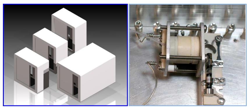
Light trapping connector between ion pump and experimental chamber. Unit is comprised of three, bonded together sub units that have blackened interiors and staggered openings to help stop radiation of various kinds from reaching the experimental unit from the ion pump.
